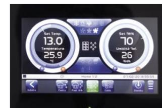
Through a touch screen panel is possible to choose four different preset programs or to adjust temperature and humidity according to the customer needs.
